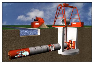
Microtunnelling with a closed front boring system for pipe jacking in inaccessible and accessible diameters (400 mm to 3,200 mm internal diameter) is highly suitable for underground crossings of rivers, roads, nature areas and other infrastructure.
