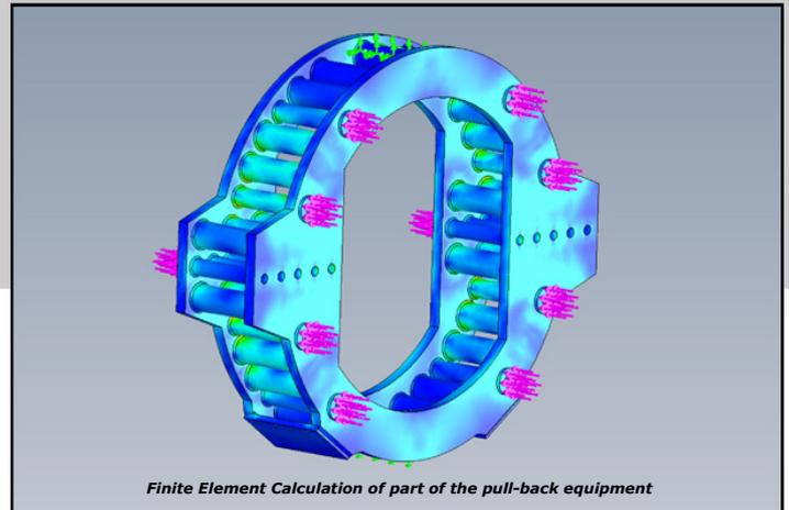
Finite Element Calculation of part of the pull-back equipment
